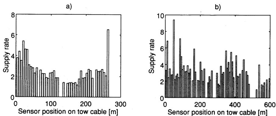
Fig. 4. Supply rates of sensors aligned on a CTD chain. A supply rate of  $n$  indicates that the sensor power supply needs only  $1/n$  of supply time to fill the storage capacitor. A missing bar means that the sensor did not respond. (a) The 270 m chain was directly coupled to the sea water at its lower end.
