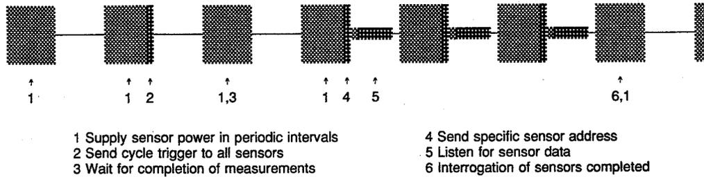
Fig. 3. Communication between deck unit and sensors. Periodic send and receive intervals are maintained during a data cycle.
